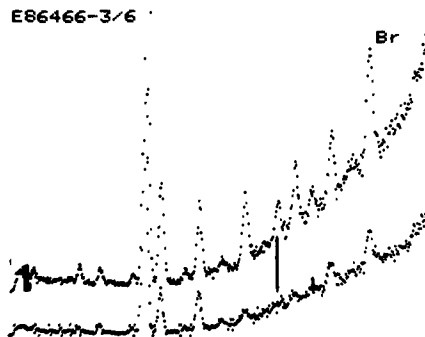
FIG. 3—Cathode-ray tube display of spectrum of the questioned sample over spectrum of the standard.
